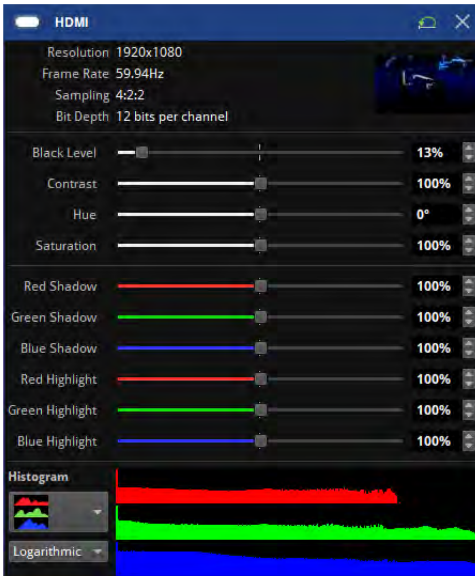
Figure 9.13 - Adjusting the black level control will make the blacks look darker and the concentrations of colour now reach down to 0% on the scale
