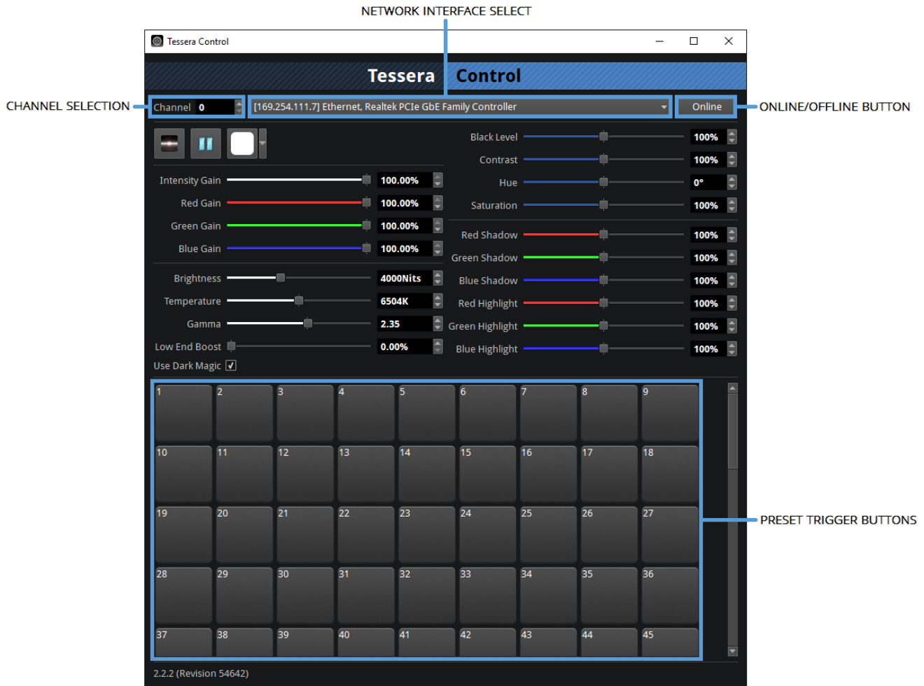
Figure 15.22 - Control application GUI
