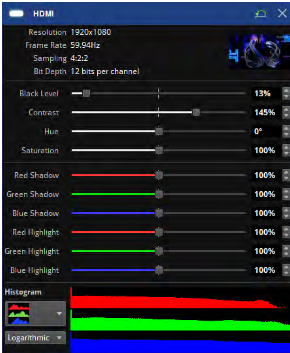
Figure 9.14 - Adjusting the contrast control will make brighter areas appear closer to the 100% threshold, assuming some areas contain white content in the image and is desirable
