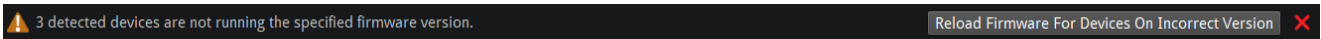
Figure 16.12 - Error message notification shown when detected fixtures are running incorrect firmware versions
