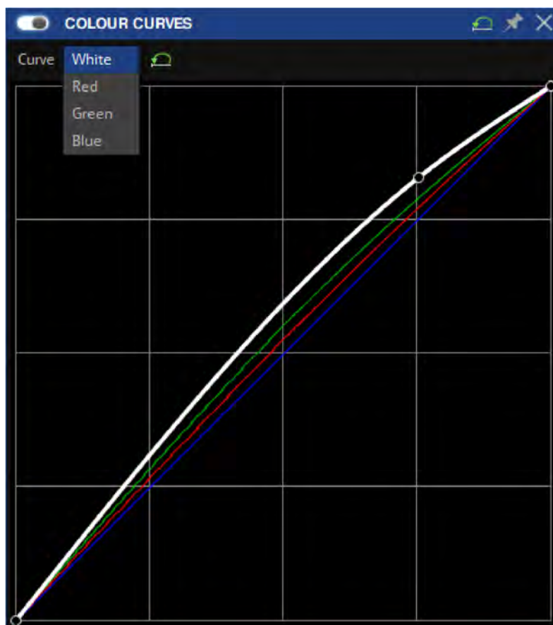
Figure 10.25 - Curves property editor, showing a colour selection drop-down menu, adjust the curves by dragging the colour curve
