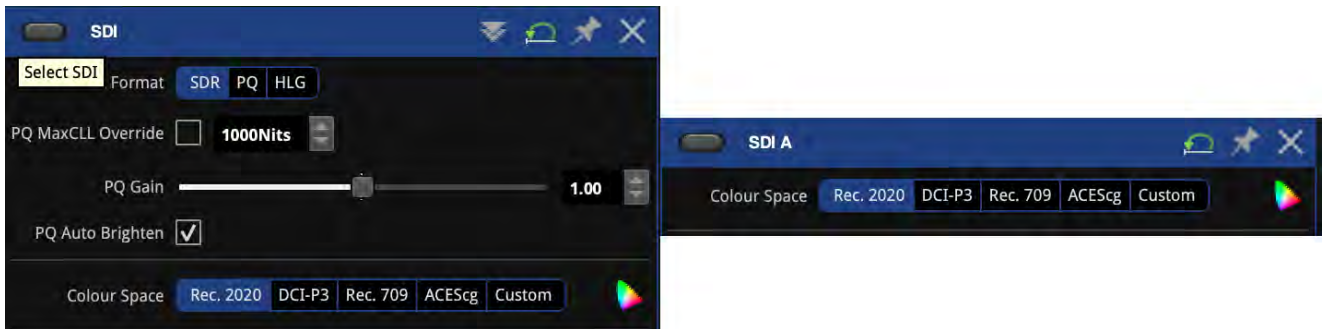
Figure 9.8 - Input override controls for SDI inputs on the Tessera SX40 (left) and M2 (right)
