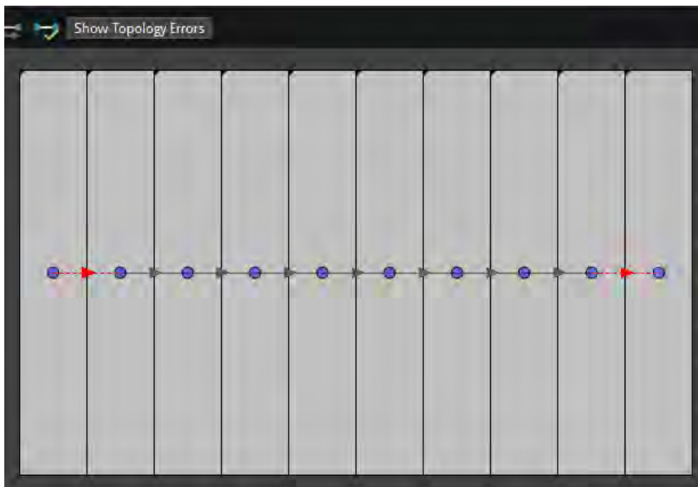
Figure 7.34 - Example of incorrect topology, notice the arrows on the far left and right are highlighted in red
